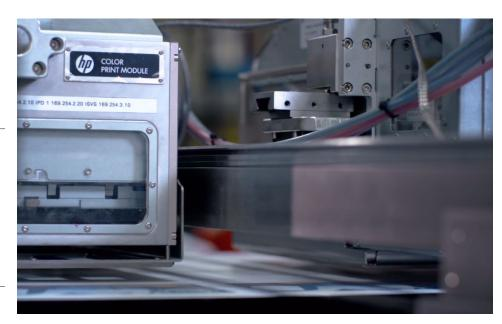
"The full color CMYK HP C800 Print Module with iDataPrint™ software features automated printhead servicing that manages purging and wiping of the print modules without having the operator manually touch the printheads. The automatic, self-contained cleaning station also eliminates messy and time-consuming start-up and shut-down procedures."
